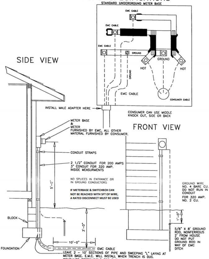
LEAVE 2 - 10' SECTIONS OF PIPE AND SWEEPING "L" LAYING AT METER BASE. E.M.C. WILL INSTALL WHEN TRENCH IS DUG.
